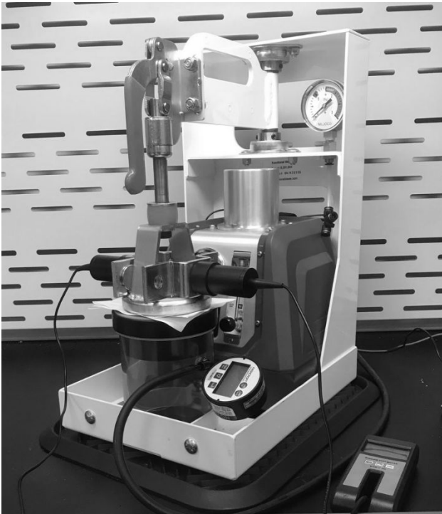
N FIGURE A.12.2.3(a) Complete QSIM Testing Apparatus.
