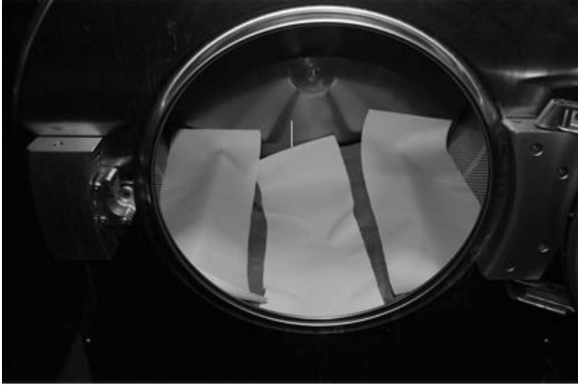
N FIGURE 12.9.3.7(b) Placement of Panel F (3 Pieces) into Washer/Extractor Drum.
